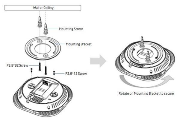
3. Mount the Access Point on the mounting bracket by rotating the unit clockwise about 90 degrees to secure it in place.
