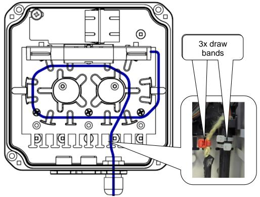
4. Fit the connector panel with SC duplex adapters without flanges (unless already fitted). Connect 1.5 m long pigtails to the adapters (unless already fitted). For inserting pigtail fibres in the cassettes, see the diagram. For easier access to the connector panel, the panel can be removed by loosening the screw.
