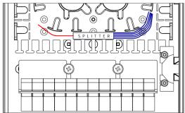
6. Fit the connector panel with adapters (unless already fitted). Connect 1.5 m long pigtails to the adapters (unless already fitted). For inserting pigtail fibres in the cassettes, see the diagram.
