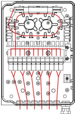
7. Splice pigtails onto the inlet cable optical fibres. The maximum length of splice protection is 45 mm. Place the splices (two in each groove of the holder one above the other) and optical fibre reserves into the cassette and replace the cassette lid. Keep the prescribed length reserves and observe the minimum bending radius of optical fibres.
