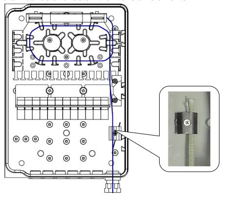
4. Remove the protective tubing from buffers along the required length, secure the tubing with a draw band and lead the fibres into the cassettes as shown.
