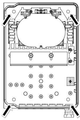
2. Using an appropriate tool, remove the outer jacket from the cable end and clean gel, if any, along at least 1.5 m. Remove the end caps from the feed-throughs and introduce the cables into the distribution box.
