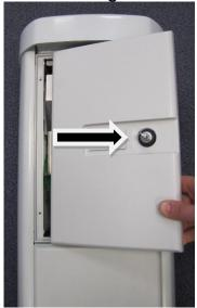
2. Remove the sliding covers located in the small pillar under the distribution box door.
