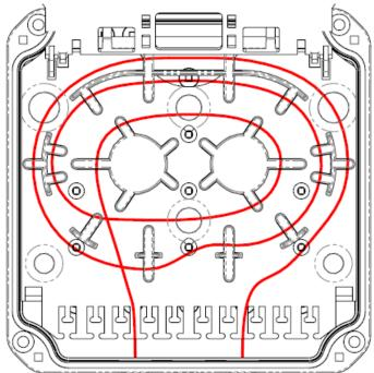
6. Linking optical fibers and splicing. Input and output fibers insert into the cassette according to the diagram. Use fiber compliant with ITU-T G.657A. Image is for illustrative purposes only.
