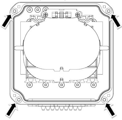
4. Bushings, insert cables or protective tube into the cabinet and attach the fastener band (see attached). Image is for illustrative purposes only.
