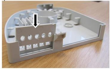
5. Choose suitable panel for connector(s). Click or screw required adapter and slide it into a bottom of ORM2.
