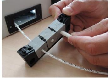
9. If bushings with inserts in two rows are used, place the top row with the smooth side down.
