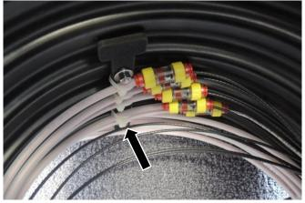
5. Attach the seal on the outside of the distribution box at the point of the bushing installation.
