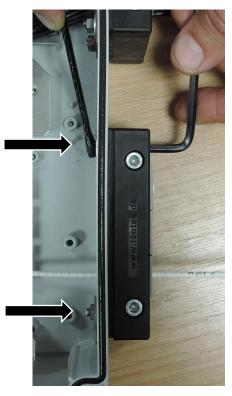
15. Assemble the holder of drop cables (see the accessory bag) as shown in the figure and fix the cables by cable ties.
