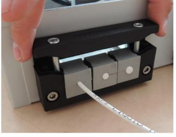
12. Fix the cables by cable ties, or attach tension elements.
