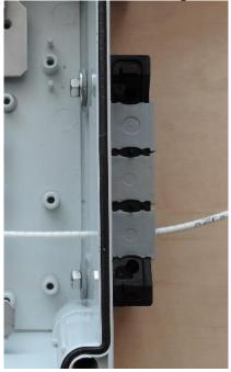
11. Install the top part of the frame. Do not tighten the screws.
