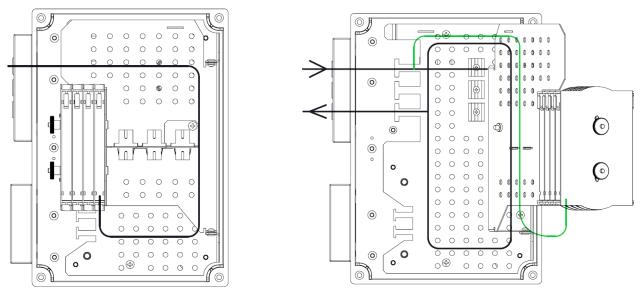
17. Insert the reserves of drop cables in the eyes and place them in the trays. If you use drop cables with connectors, plug them into the adapters and place the fibre reserves in the trays.
