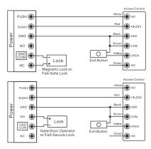
Attention: A 1N4004 or equivalent diode is needed when use a common power supply, or the reader might be damaged. (1N4004 is included in the packing)
