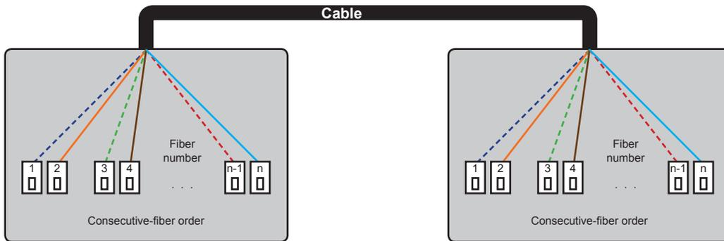
*Reverse-pair positioning.* Fibers are arranged consecutively (e.g. 1-n) on one end of the link, but each duplex pair is reversed on the other end (i.e. 2,1 4,3 6,5 etc.). Behind the patch panel, the consecutive-fiber side connectors are installed “keys up” while the reverse-pair side connectors are installed “keys down”.
