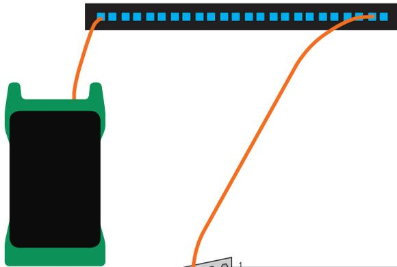
...or measure the transmitter power through the link.
