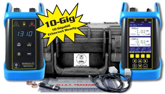
**Power Meter:** Fiber OWL 7X (p/n: F7X) **Light Source:**WaveSource Pro SM/VFL (p/n: WPSV) Patch cables, adapters, and other related accessories not included.
