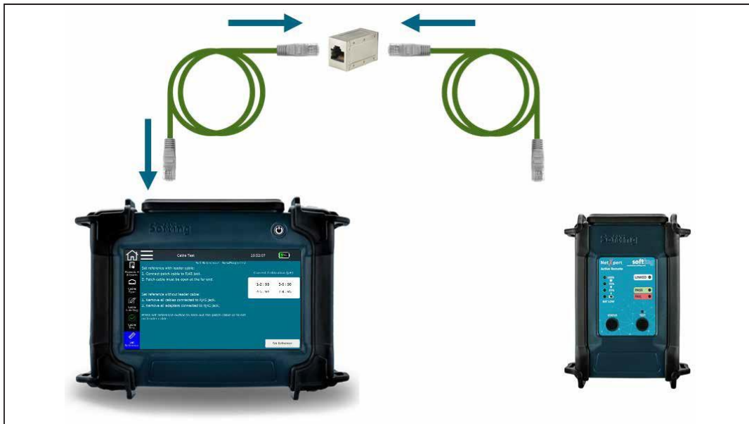
Figure 39 - Test setup for setting the reference - Cu
