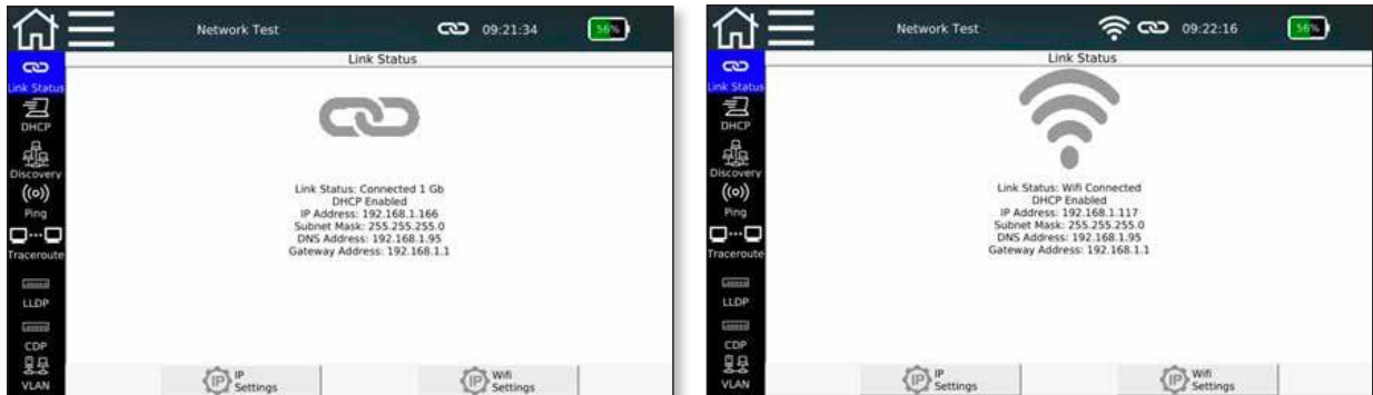
Figure 43 - Link Status, wired connection {left} or via WiFi {right}
