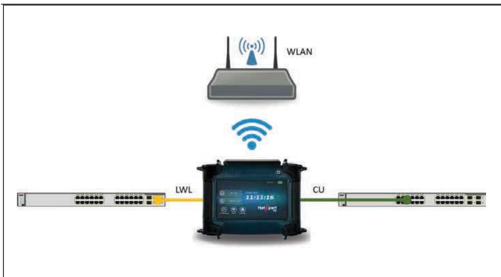
Figure 42 - Test setup for connecting to an active network
